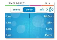
User interface with virtual add-on. 4 programmable softkeys are displayed and can be used as a smart add-on module.
